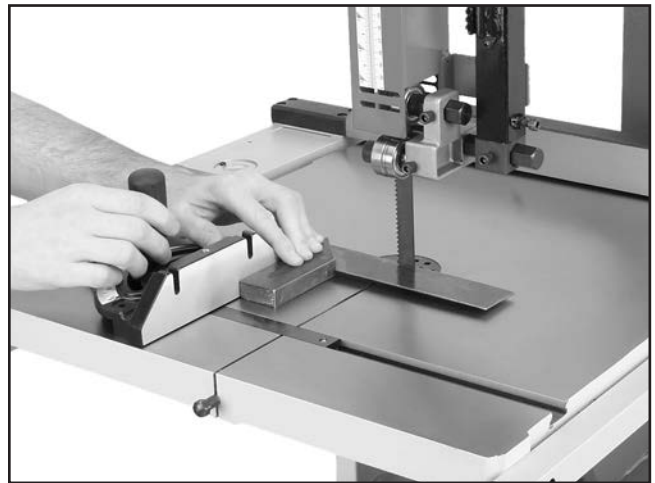
Figure 31. Squaring miter gauge to blade.
