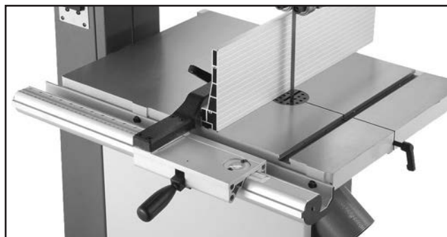
Figure 15. Correctly installed fence.
